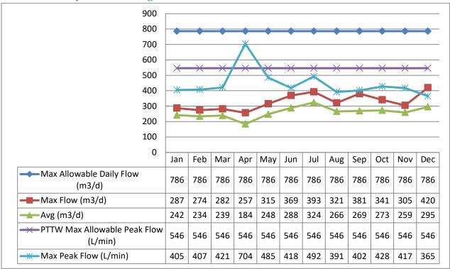
The Peak Flow rate was increased in May 2020 during scheduled flow meter calibrations.
