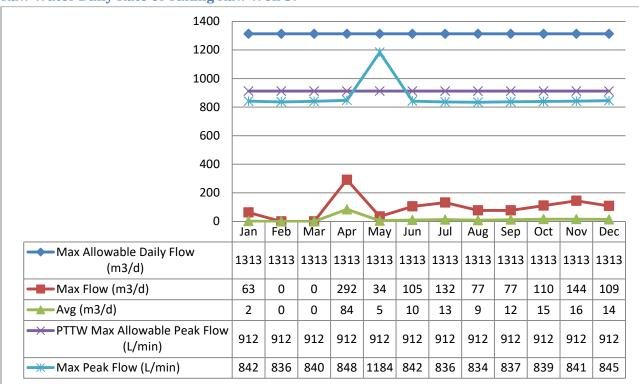
The Peak Flow rate was exceeded in May 2020 during scheduled flow meter calibrations.
