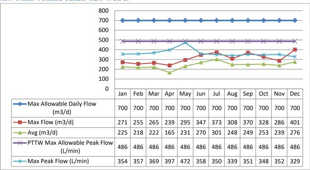
The Peak Flow rate was increased in May 2020 during scheduled flow meter calibrations.
