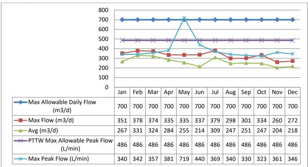
The Peak Flow rate was increased in May 2019 during scheduled flow meter calibrations.
