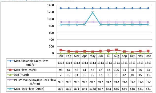
The Peak Flow rate was exceeded in May 2019 during scheduled flow meter calibrations.
