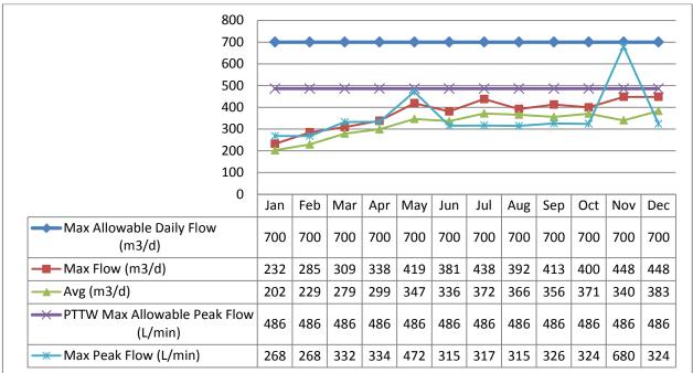
The above table shows there was an exceedance in November 2015 for instantaneous peak flow rate (L/min), this occurrence was due to maintenance during the Raw Well 1 pump replacement.
