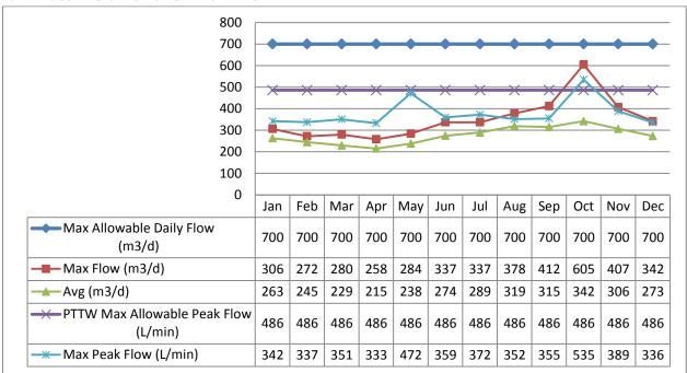
The Peak flow rate was exceeded in October 2017 due to hydrant flushing maintenance.
