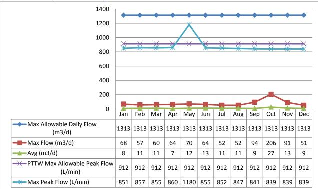
The Peak Flow rate was exceeded in May 2017 during scheduled flow meter calibrations.
